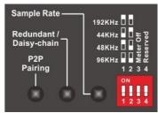
• **P2P Pairing** button: long-press the button for longer than 2 seconds or until a SET shown on the meter panel, the NBB-1616 enters P2P (peer-
