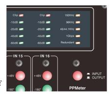
Besides measuring input audio, you are able to switch all the 16 meters to monitor level on output by simply pressing an INPUT/OUTPUT button on the far right of the front panel.
