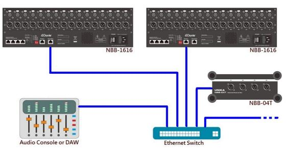
**System Scaling Up** Computer network can be further expanded with more than one Ethernet switch, so does NBB-1616 audio network. You can use more than one switch between NBB-1616s to greatly expand your audio distribution.
