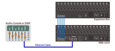
**Daisy-chain** With the two network ports configured to work in switch mode, you can cascade several NBB-1616s in a same link. This greatly simplifies the network wiring and devices deployment if you need to route audio to several spots sequentially.
