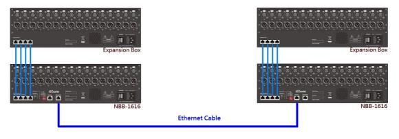
**Stagebox** With a Dante-enabled audio console, you can have the NBB-1616 to work as a stagebox. The console can then route multi-channel audio to/from NBB-1616 on remote site with a single Ethernet cable. Similarly, you can also have your DAW software to transceive multi-channel audio to/from NBB-1616 if your DAW software also supports Dante networking or if you have Dante Virtual Soundcard installed along with your DAW software.
